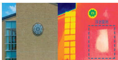
Can detect unevenness in tiles that cannot be detected by visual inspection
