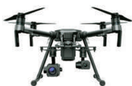
Inspection drone equipped with an infrared camera
